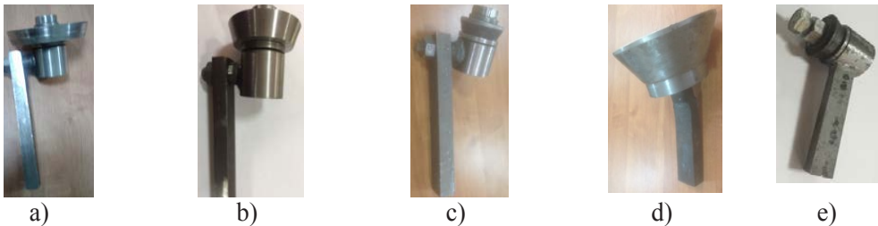
a – cup cutter made of HARDOX steel; b - cup cutter made of 65Г; c,e - cup cutter made of 20X; d - cup cutter made of DI40 (Ductile iron)
